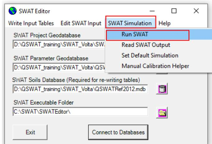
Figure 14. Step to defining and running the SWAT simulation
