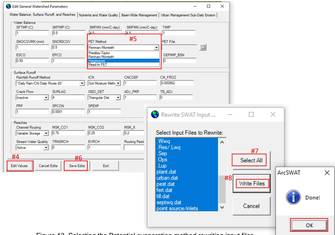
Figure 13. Selecting the Potential evaporation method rewriting input files
