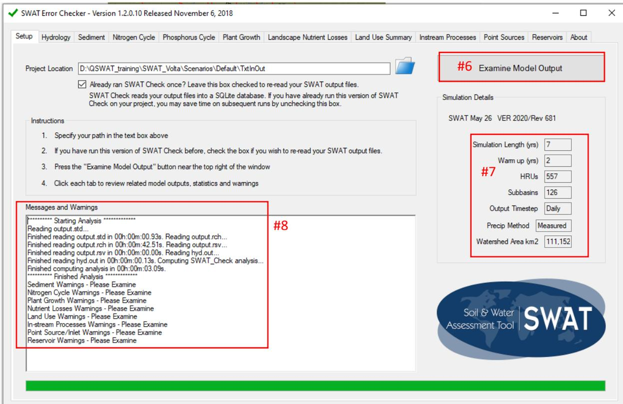
Figure 19. Steps to running SWAT checks
